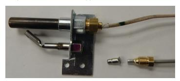
Remove the main burner orifice and replace with LP main burner orifice supplied in conversion kit. Set Air Shutter to full open before reinstalling Brass Elbow.
